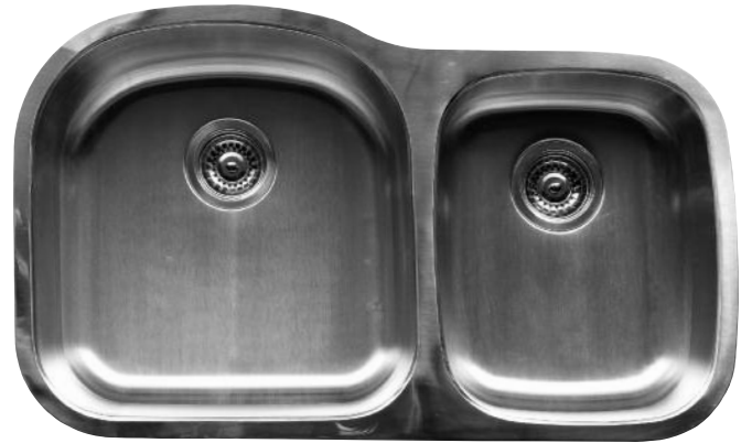
Model: L-UM12R Outside dimensions: 33 7 / 8 " x 20 1 / 2 " Inside bowl dimensions: Left bowl: 17 5 / 8 " x 18 3 / 8 " x 9" Right bowl: 13" x 16 1 / 4 " x 7" Gauge: 18
